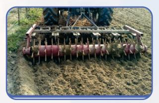
The length of the clod crusher is a foot more than that of the cultivator to provide a better coverage area. The machine covers 0.32 ha per hour, consuming 3.5 litres of diesel.
